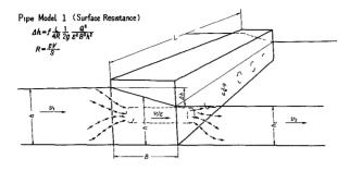
Fig 1 Resistance-pipe model
