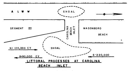
A schematic flow diagram of the computed average annual littoral process at the inlet is given in Diagram 5
