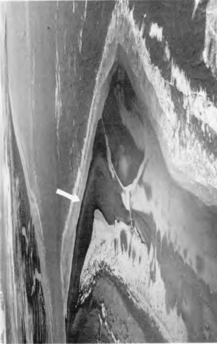
Fig. 5 Offset coastal inlet, Copper River Delta, Alaska. View is toward the east. Note the large seaward protrusion on the downdrift (west) side of the inlet with the linear beachface (arrow) perpendicular to the southeast, the dominant wave approach direction.
