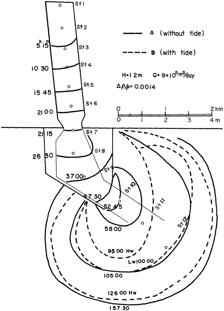
Fig. 12 Change of area with time of dyed water from a continuous point source (model)
