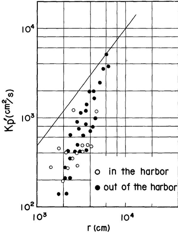
Fig. 9 Diffusivity  $K_p'$  and equivalent radius  $r$  in presence of the tide (model)<sup>p</sup>
