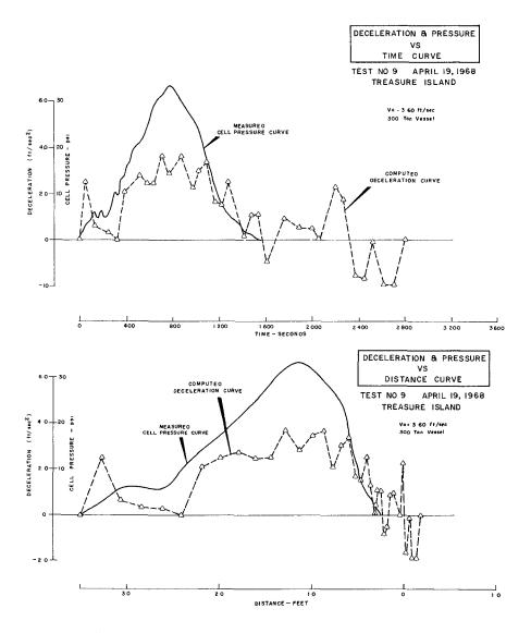
Figure No 7 - A comparison of time and distance curves for Test No 9- Hi-Dro Cushion Camel.
