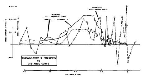
Figure No. 8- Test No 15, May 13, 1968, Treasure Island. Comparison of pressure distribution between adjacent clusters
