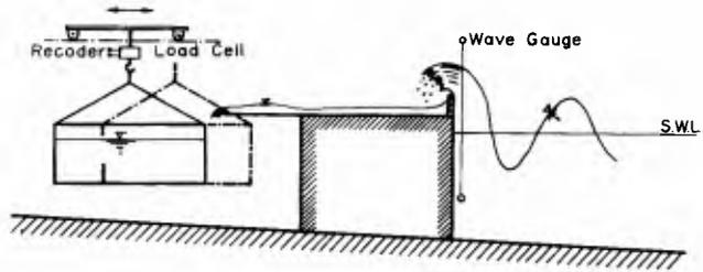
Fig. 3 Experimental set-up for the measurement of wave overtopping
