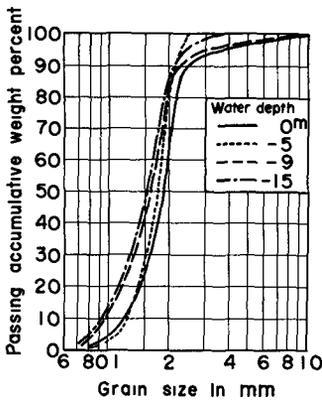
Fig. 10. Typical accumulative curves of grain size.
