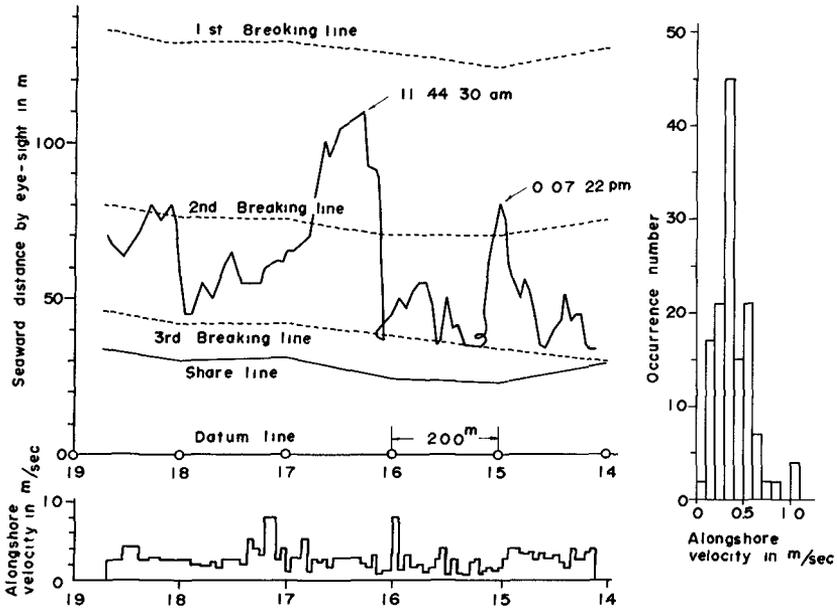
Fig. 14. An example of longshore current diagram.
