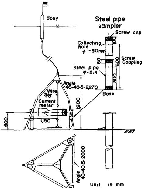
Fig. 5. Self-recording current meter attached with steel pipe samplers.
