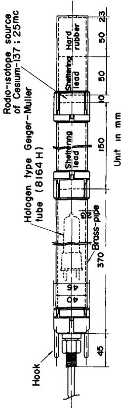
Fig. 20. Detection pick-up of the scouring meter.
