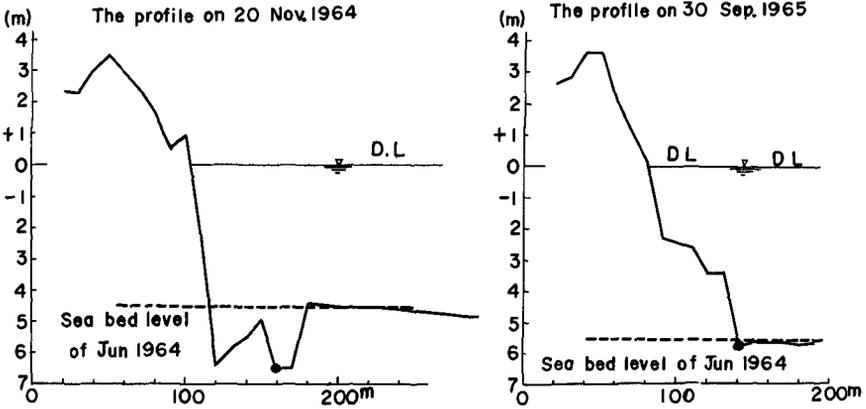
Fig. 16. Scoured hollows at the tip of breakwater.
