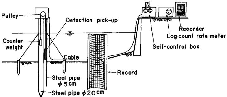
Fig. 19. Self-recording scouring meter.
