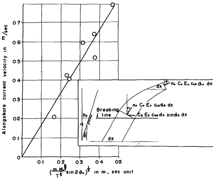
Fig. 15. Relation between longshore current velocities and characteristics of deep water waves.
