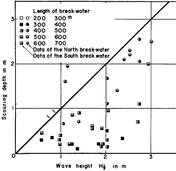
Fig. 18. Relation between wave height and scouring depth.
