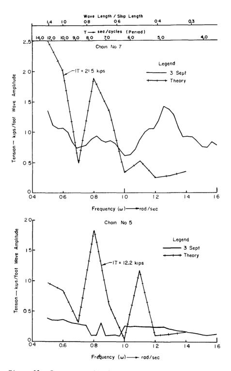
Figure 11. Response amplitude operator for port and starboard quarter chains (#7 and #5).
