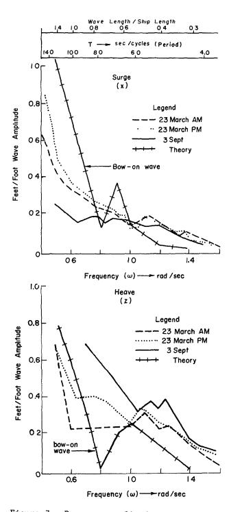
Figure 7. Response amplitude operator for surge and heave.
