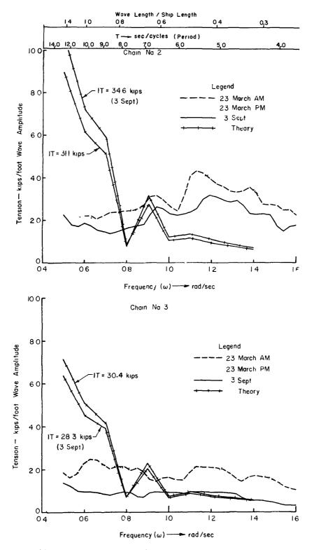
Figure 10. Response amplitude operator for port and starboard bow chains (#2 and #3).
