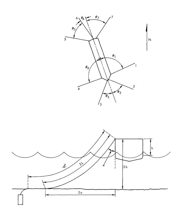
Figure 2 Convention used to describe mooring chain geometry. (See Table II for actual dimensions and tensions.)
