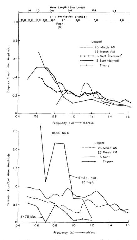
Figure 8. Response amplitude operator for pitch and stern chain (#6).
