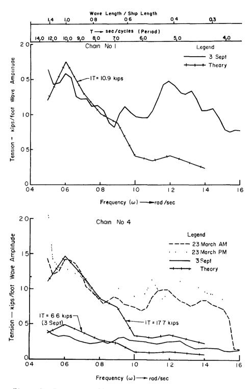
Figure 9. Response amplitude operator for port and starboard breast chains (#1 and #4).
