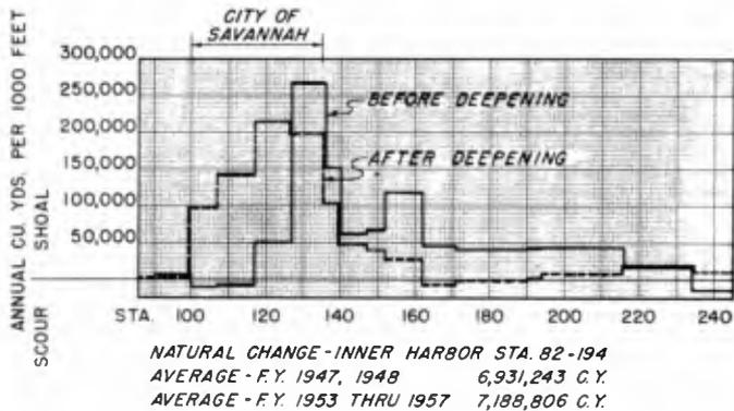
FIG. 2 - ANNUAL SHOAL AND SCOUR (NATURAL CHANGE) BEFORE AND AFTER DEEPENING NAVIGATION CHANNELS
