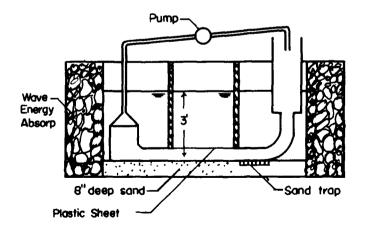
FIG. 11. CROSS SECTION OF WAVE TANK FOR TESTS ON BED-LOAD TRANSPORT BY WAVES PERPENDICULAR TO CURRENTS
