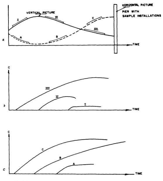
FIG 3 INTERFERENCES BY MIGRATING WAVES WITH LONGSHORE BED-LOAD TRANSPORT (c=CONCENTRATION OF TRACER MATERIAL)
