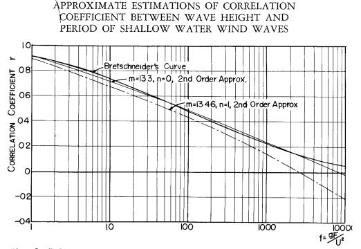
Fig. 1. Relation between correlation coefficient and non-dimensional fetch for deep water waves.
