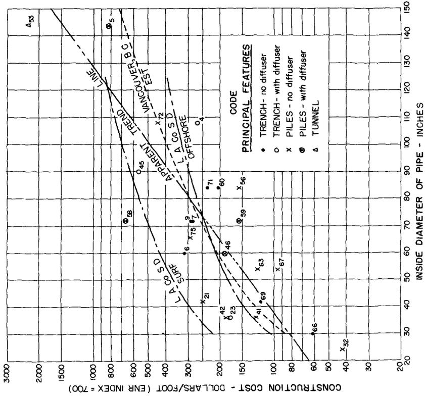
Fig. 8. Construction costs of reinforced concrete submarine outfalls
