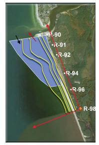
Figure 12. Schematic of NLINE model coverage for downdrift beach evolution modeling
