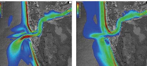
Figure 7. Wave and current interaction at ebb and flood tidal stages for the 2000's conditions
