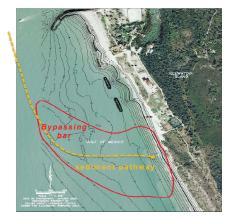
Figure 16. Proposed design, beach response and inlet sand bypassing
