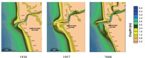
1957 2008 Figure 2. Gordon Pass bathymetry at various temporal stages
