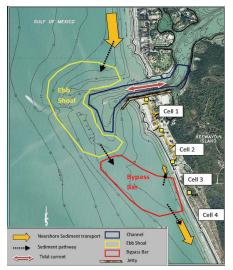
Flow due to waves and flood tidal currents
