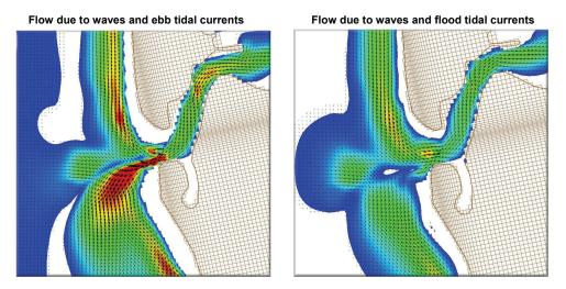
Figure 5. Wave and current interaction at ebb and flood tidal stages for the 1930's conditions
