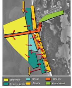
Figure 9. Schematic of IRM model setup for Gordon Pass
