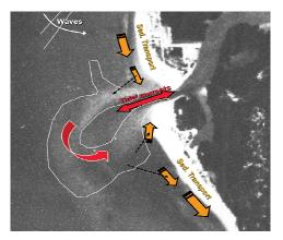
Figure 6. Schematic of sediment pathways for the 1930's conditions
