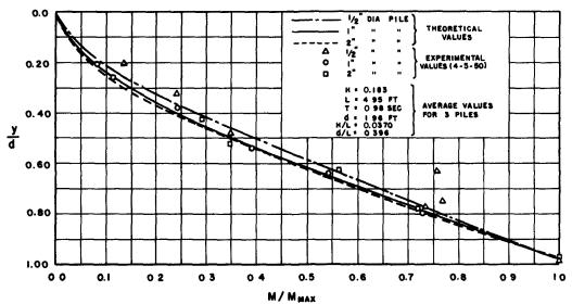
Fig. 5. Dimensionless moment distribution of uniform pile.
