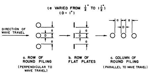
Fig. 11. Arrangement of piling for tests on mutual interference.
