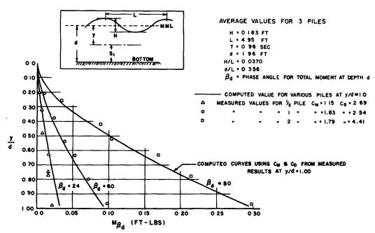
Fig. 4. Moment distribution on uniform pile - Laboratory results.
