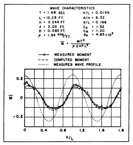
Fig. 3. Total moment about the bottom of a single circular pile.
