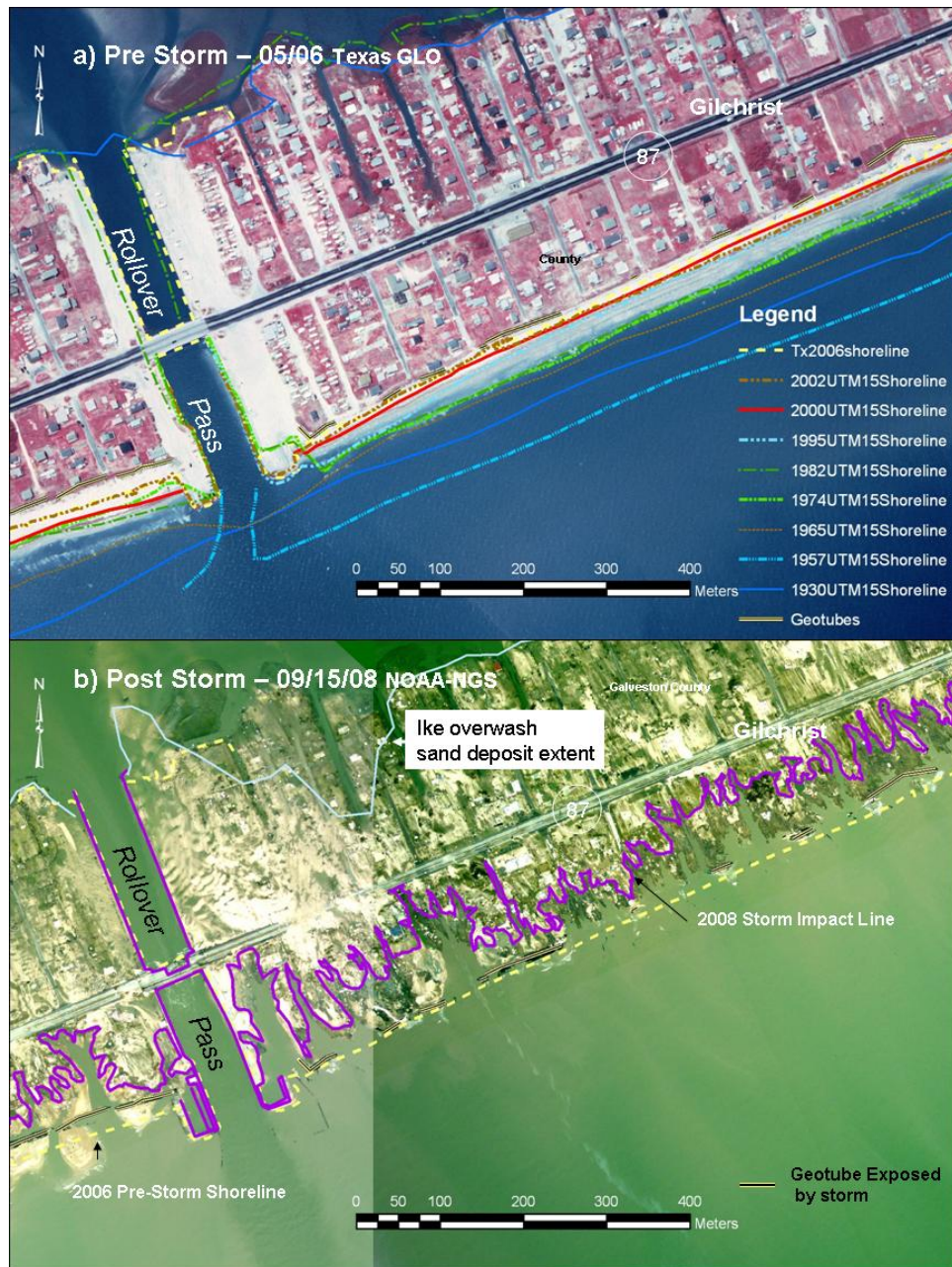
Figure 8 (a) Pre-storm aerial photography of Rollover Pass and Gilchrist with historic shorelines and location of buried geotextile tubes and (b) post-storm impacts of overwash extent and shoreline position
