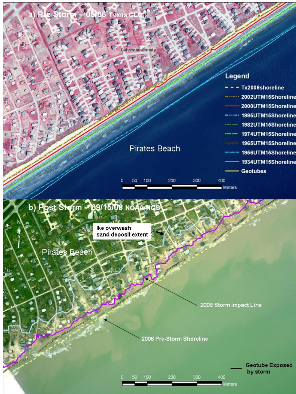
Figure 9 (a) Pre-storm aerial photography of the Pirates Beach area of West Beach showing the historic shorelines and dune over geotextile shore protection and (b) post-storm impacts to geotextile tubes, overwash extent, and shoreline position
