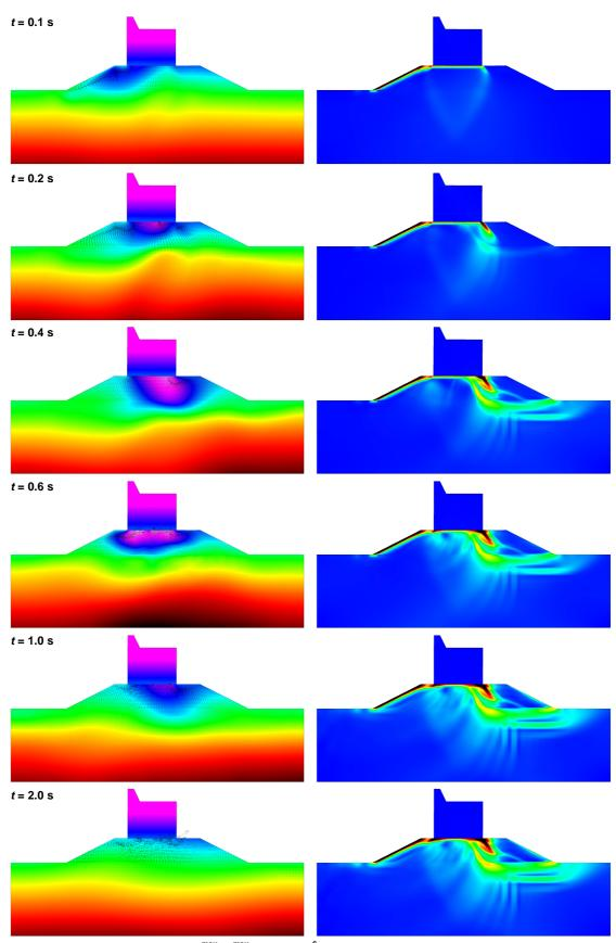
Figure 13. Results for  $t_1 = 0.2$  s;  $P_2^{max}/P_1^{max} = 8$ ;  $k = 10^{-6}$  m/s. Left: Pore pressures; the color range goes from magenta (p = 0 Pa) to dark red (p = 600 kPa); white shades indicate negative pressures and arrows show the flow. Right: Plastic strain magnitude (dark red shades indicate large deformation).
