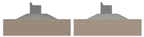
Figure 7. Geometry applied in the numerical models. Left: Finite elements with linear spatial interpolation in ABAQUS and cells used in FLAC. Right: Finite elements with quadratic spatial interpolation in ABAQUS.
