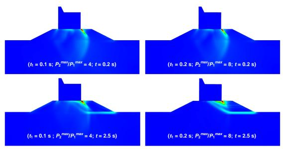
Figure 10. Deformations due to wave impact in the non-porous FLAC model at two different magnitudes of the load and two different times. Dark, red shades indicate large plastic strain magnitudes, whereas blue shades correspond to no plastic deformation.
