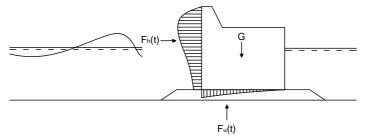
Figure 2. Dynamic part of the hydraulic pressure distribution from wave slamming on a caisson.
