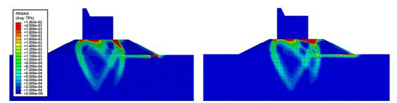
Figure 9. Failure mechanism under static loading obtained by ABAQUS. Left: Linear spatial interpolation. Right: Quadratic spatial interpolation. The color scale indicates the plastic strain magnitude.
