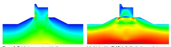
Figure 8. Total stresses at rest in the non-porous model obtained by FLAC. Left: Vertical normal stresses; the color range goes from dark brown ( $\sigma_{zz} = -1000$  kPa) to blue ( $\sigma_{zz} = 0$  MPa). Right: Horizontal normal stresses; the color range goes from dark brown ( $\sigma_{xx} = -200$  kPa) to blue ( $\sigma_{xx} = 40$  kPa).
