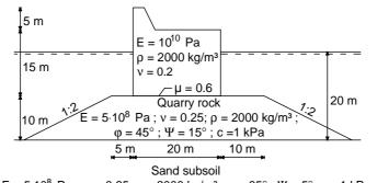
$E = 5 \cdot 10^8 Pa ; v = 0.25; \rho = 2000 kg/m^3; \phi = 35^\circ; \Psi = 5^\circ; c = 1 kPa$ Figure 4. Geometry and material properties of the considered caisson, rubble foundation and seabed.
