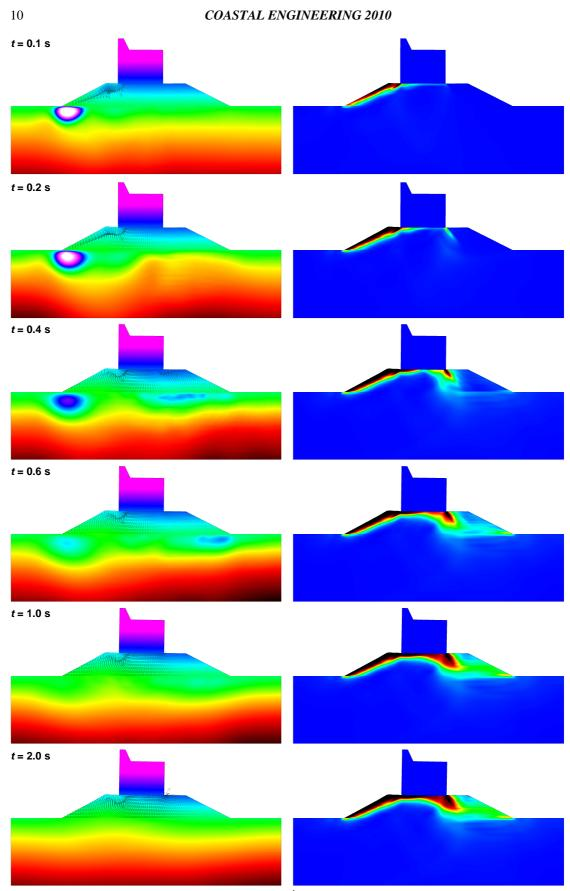
Figure 12. Results for  $t_1 = 0.2$  s;  $P_2^{max}/P_1^{max} = 8$ ;  $k = 10^{-4}$  m/s Left: Pore pressures; the color range goes from magenta (p = 0 Pa) to dark red (p = 600 kPa); white shades indicate negative pressures and arrows show the flow. Right: Plastic strain magnitude (dark red shades indicate large deformation).
