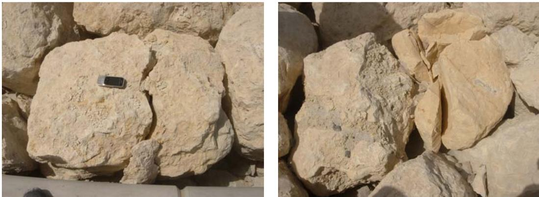
Figure 3. Examples of rocks which have been broken during placement.
