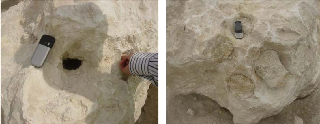
**Figure 1. Examples of rocks containing voids (left) and clay pockets (right).**
