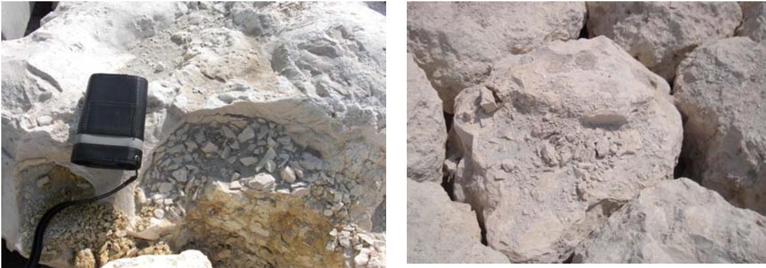
**Figure 2. Examples of rocks showing surface crumbling after approximately three years in service.**
