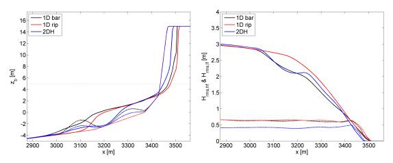
Figure 8: Left panel: longshore averaged pres-storm profiles (dotted lines) and post-storm profiles (solid lines). Right panel: longshore averaged transformations of short waves (solid lines) and long waves (dotted lines).
