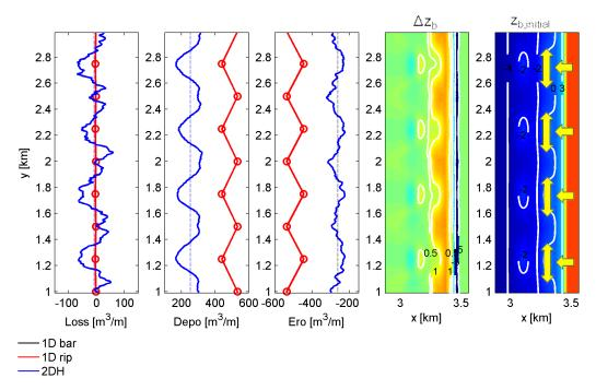
Figure 9: Simulations results as function of longshore distance including from left to right, the alongshore sediment loss, deposition volume below maximum storm surge level, dune erosion volume above maximum storm surge level, erosion deposition pattern and the initial bathymetry.
