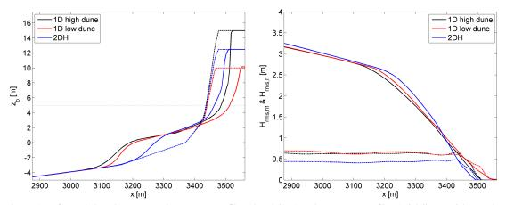
Figure 5: Left panel: longshore averaged pres-storm profiles (dotted lines) and post-storm profiles (solid lines). Right panel: longshore averaged transformations of short waves (solid lines) and long waves (dotted lines).
