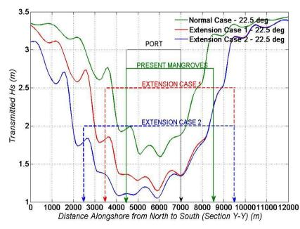
Figure 11: Wave heights at port for original mangroves and the two extension cases at 22.5 deg wave attack angles for a 25 year event. The solid black lines indicate the position of the port, the solid green lines the existing extent of mangroves and the dotted red and blue lines the extent of mangroves for extension cases 1 and 2 respectively
