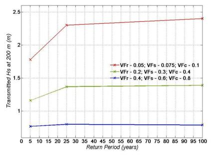
Figure 6: Transmitted wave heights at 200 m forest width for different vegetation factor values and different input wave heights for increasing return periods (constant h = 9.6 m and Tp = 15 s)
