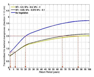
Figure 10: Wave heights at the port at a point directly behind the mangroves versus return periods for different cases of vegetation
