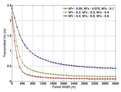
Figure 4: Transmitted wave heights across forest width for varying vegetation factor values for roots (VFr), stems (VFs) and canopies (VFc) with constant hydraulic parameters (h=9.6m. Hs=2.5m, Tp=15s)
