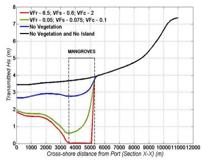
Figure 9: Transmitted wave heights from offshore (right) along Section X-X (cross-shore) for different vegetation factors compared with the 'no veg. and no island' case for a 25 year event
