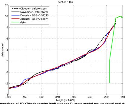
Figure 4. Comparison of 1D XBeach results (red) with the Durosta model results (blue) and the measured bathymetry (black) for section 116.
