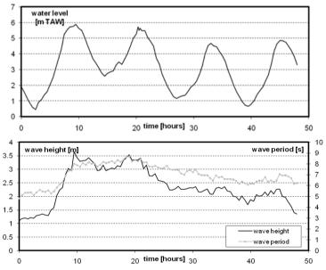
Figure 3. Hydrodynamic conditions at Ostend "noodstrand" buoy during the November 2007 storm.
