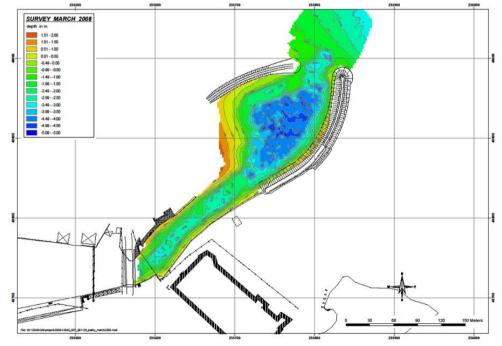
Figure 9. Bathymetry after construction of the breakwaters and dredging inside Elmina harbour (March 2008).
