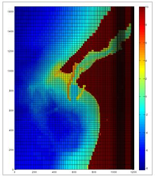
Figure 11. Grid of the Elmina 2D XBeach model. The colour scale shows the bathymetry [m LAT].
