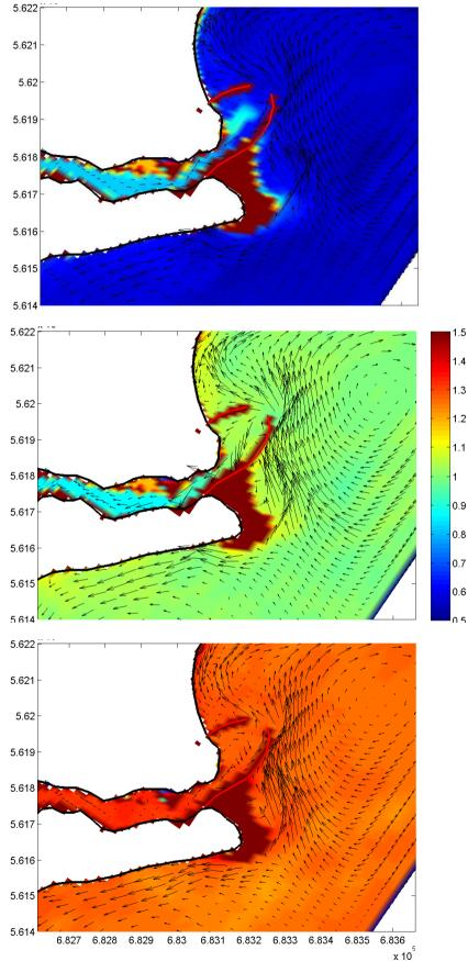
Figure 12. Current pattern due to tide and waves during ebb (arrows), on the background the water level (colour scale, m LAT). On top: low tide; in the middle: rising tide; at the bottom: high tide.
