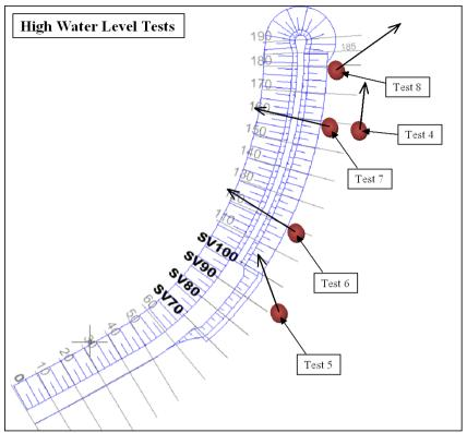
Figure 17. Result of the dye tests performed at high water.
