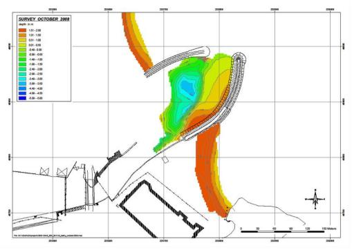
Figure 10. Bathymetry half a year after construction of the breakwaters and dredging inside Elmina harbour (October 2008).
