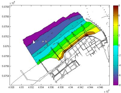
Figure 2. Bathymetry in front of Ostend city centre (depths in m TAW).
