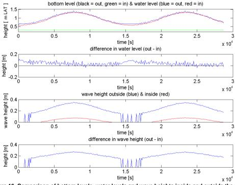
Figure 16. Comparison of bottom levels, water levels and wave heights inside and outside the main breakwater for cross-section A-C.
