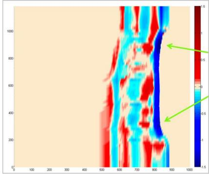
Figure 6. 2D erosion (blue) / sedimentation (red) pattern for Ostend beach, caused by the November 2007 storm event.
