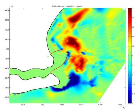
Figure 14. Erosion (blue) / sedimentation (red) pattern [m].
