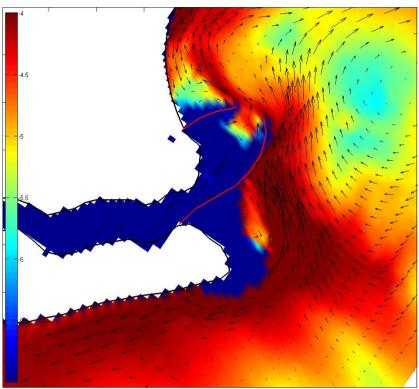
Figure 13. Current pattern due to tide and waves during ebb (arrows) with on the background the sediment concentration (in colour, on a log scale).
