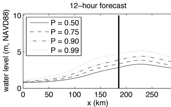
Figure 2. Surge forecast for Hurricane Ike (2008) at 12 hours from landfall. Horizontal axis is alongshore position, measured from the southwestern end of Matagorda Bay (see Figure 1). Vertical line indicates actual landfall position of Hurricane Ike in Galveston, Texas (modified from Irish et al. in review).
