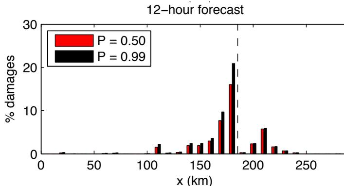
Figure 3. Damage forecast for Hurricane Ike (2008) at 12 hours from landfall. Horizontal axis is alongshore position, measured from the southwestern end of Matagorda Bay (see Figure 1). Percent damages represents percent of entire value for the stretch of coast from Matagorda Bay, Texas to the Texas/Louisiana border. Vertical dashed line indicates actual landfall position of Hurricane Ike in Galveston, Texas.
