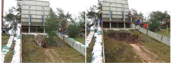
Figure 7. Dike slope after 4 hours of 10 I/s per m (left) and after that 30 minutes of 20 I/s per m, the 7-cmdiameter casuarina collapsed (right).
