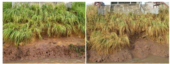
Figure 18. Vetiver grass slope at location DS\_01. Left: after 4 hours of 20 l/s per m and 1 hour of 40 l/s per s. Right: final situation.
