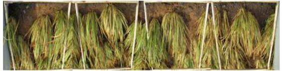
Figure 13. Clumps of Vetiver grass remained intact during testing.
