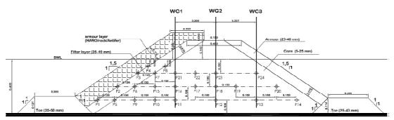
Figure 2. Cross section of the breakwater model (dimension are in m)
