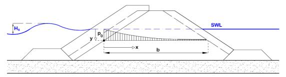
Figure 1. Definition sketch of attenuation of pore pressure height within the core of a rubble mound breakwater
