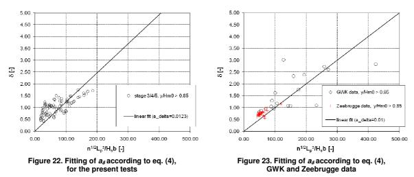
The values of the damping coefficient from the GWK dataset show a considerable scatter for large values (>100) of the dimensionless predictor. The quality of the regression analysis is generally rather poor, as can be seen from the values of the coefficient of determination given in Table 3. The coefficient of determination is defined as unity minus the proportion of the regression sum of squares to the total sum of squares.
