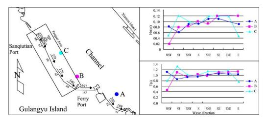
Figure 12. Pr oject area along east coast in Gulangyu Island. Points A, B and C show the wave calculation points. Wave conditions in different locations are showed on left. Longshore sediment transport  $(m^3/a)$  for each stretch is listed along the coastline.
