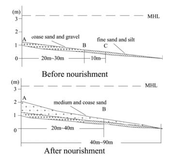
Figure 13. Beach profile design and sediment fill.
