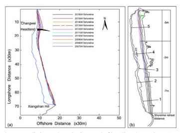
Figure 4. Shoreline change prediction and monitoring result. Shoreline change from 2007 to 2016 is shown in Panel a (left), shoreline retreat for the first winter half year is shown in Panel b (right). Numbers indicate positions of monitoring profiles.
