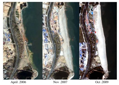
Figure 6. Comparison of satellite images of nourished beach at different time.
