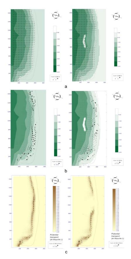
Figure 9. Comparison of wave field, longshore current and longshore sediment transport before and after the construction of submerged breakwater.a.wave height increase and direction change due to wave diffraction induced by submerged breakwater,b.currents converge from different directions behind the breakwater, c.sediment was transported from opposite directions and should deposit behind the breakwater.
