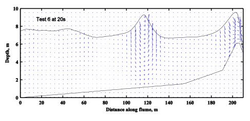
Fig. 4 A snap shot showing wave surface elevation, embankment detail and flow field velocity vectors plotted at every fifth node vertically and every tenth node horizontally.
