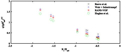
Fig. 13 Dimensionless discharge and dimensionless negative freeboard for the RANS-VOF test and calculated values based on Rc evaluated in accordance with BS3846 and a Cd value of 1.1126.
