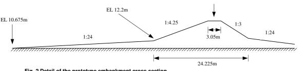
Fig. 2 Detail of the prototype embankment cross section.
