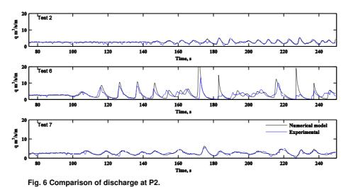
Although the general agreement is very good the RANS-VOF model has slightly larger peaks, particularly at the larger wave height (Test 6). It also shows a slight phase shift for some of the peaks and a couple of peaks showing substantial differences. This could be a result of differences in either the surge depth or velocity measurement or both. To investigate this further a comparison of time histories of surge depth and velocity in each model has been performed.
