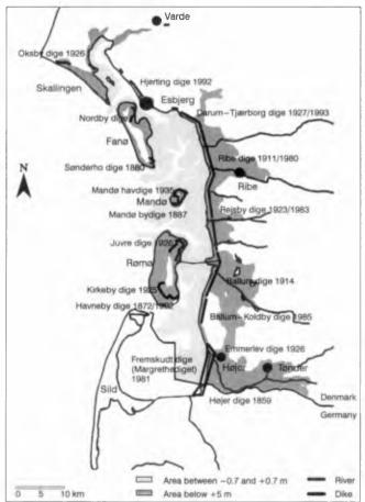
Figure 2. Upgrading of the dike system along the Danish Wadden Sea.
