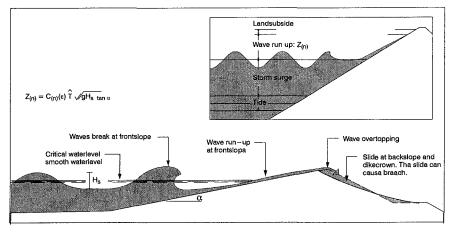
Figure 6. Design of dike height.
